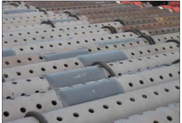
The predrilled liner with the centralizers is for Chevron's North Sea Alba field (Fig. 4).
