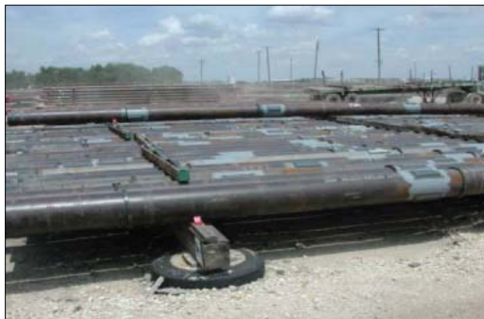
The carbon-fiber blades are on 11 \frac{7}{8} in. stress-keel joints for BP Plc's 15 well Holstein project in the Gulf of Mexico (Fig. 2).
