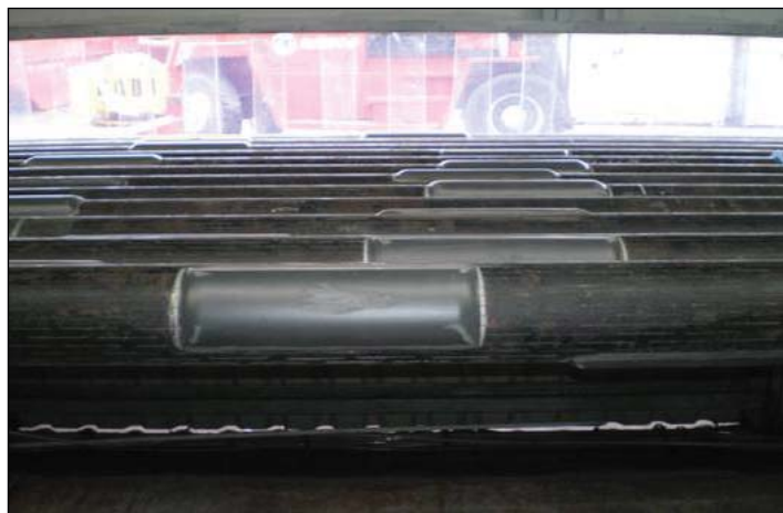
The slotted liner includes molded carbon-fiber centralizers (Fig. 1).
