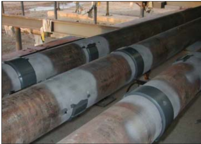
Eni Petroleum's K-2 Gulf of Mexico development included 7¾-in. pipe inside of an 8.50-in. hole opening into a 9⅞-in. section. The centralizers have a blade shape (Fig. 3).
